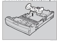
Press "Push", and then adjust the rear guide to the paper size you want to load.
