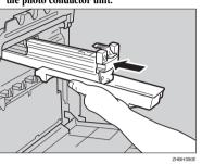
Repeat steps # to # to install the color photo conductor unit.
