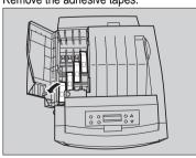
Check the toner color and location are correct, and then insert the toner cartridge vertically and
