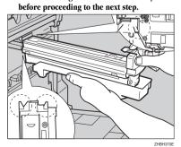
Push the front of the photo conductor unit slowly. slide the unit on the cover, and then push the unit in until it clicks.
