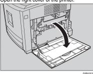
Pull out the green levers on the left and right that are fastening the inner cover, and then unlock.
