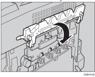
Push the green lever to fasten the inner cover.
