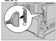
Attach the other end of the parallel cable to the port of the computer. Secure the cable.
